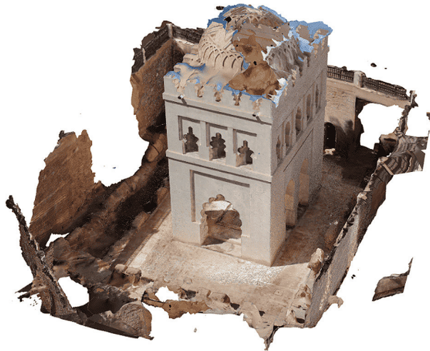
FIGURE 6 Blueprint of the Qubba generated using 3D scanner app on an Ipad Pro NOTES Left: blueprint obtained from 3D LiDAR scanning; right: plan after post-production.
